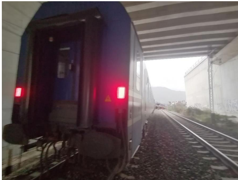
Figure 89. Positions 6-9) B4-B7 coaches, B4 and B5 derailed and were hit on the side by steel plates, B6 and B7 did not derail, no damage, B7 remained nearly all in the tunnel.
