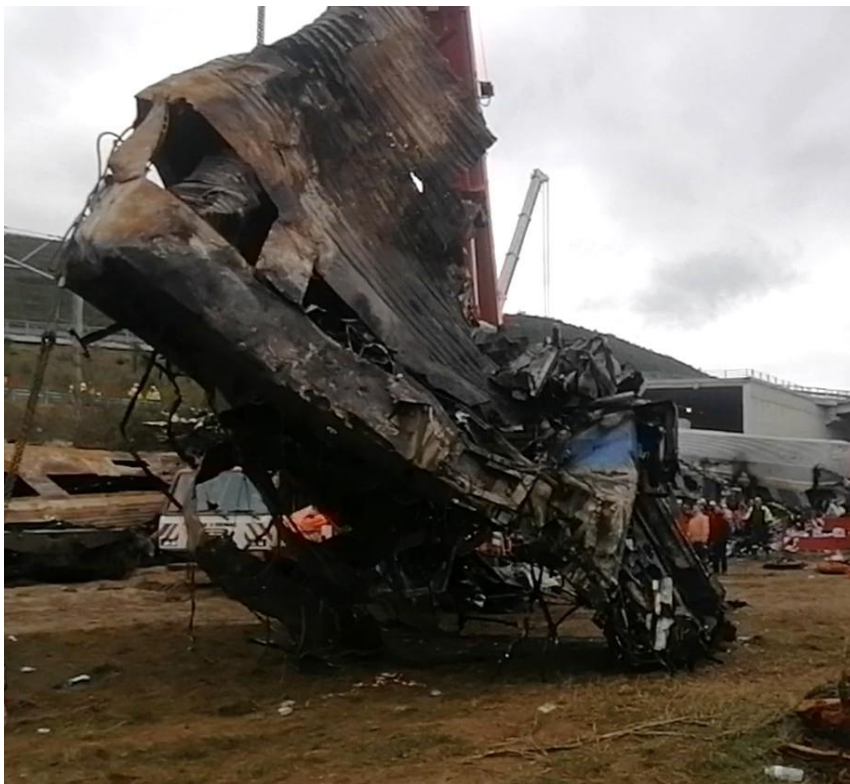
Figure 86. Position 3) Restaurant Car, very heavily damaged from initial crash (folded, bent into S-shape) and burned down. Here, suspended from the crane cables.
