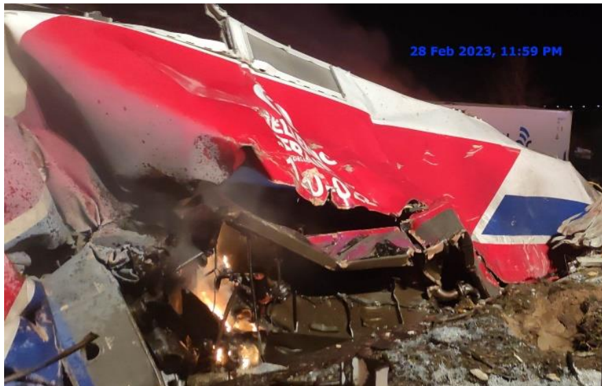
Figure 65. A local fire inside and outside the broken transformer of the first locomotive of the freight train, 40 minutes after the accident.
