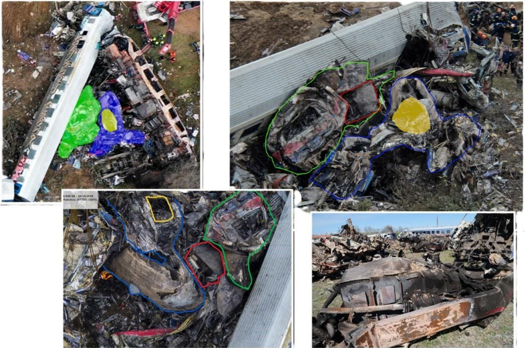
Figure 61. Further images of the location of the Restaurant Car, Passenger Locomotive and its transformer.
